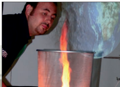
The 'bin engine' simulates the cyclonic action of a liquid fueled rocket engine
